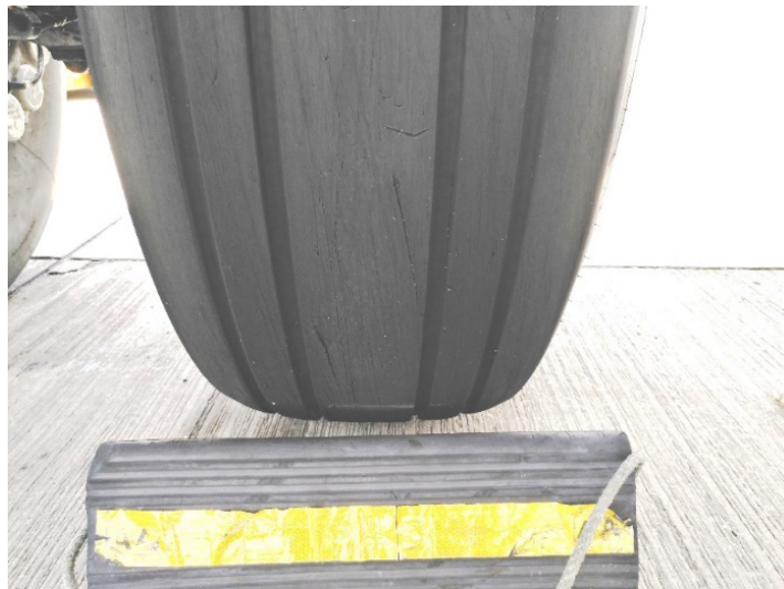
Photo 4: Significant Longitudinal Scratch Marks on No. 3 Tyre
