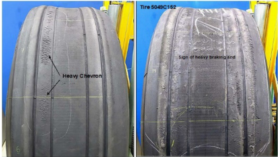
Figure 22: Damage on No.2 Tyre (Cont'd)
