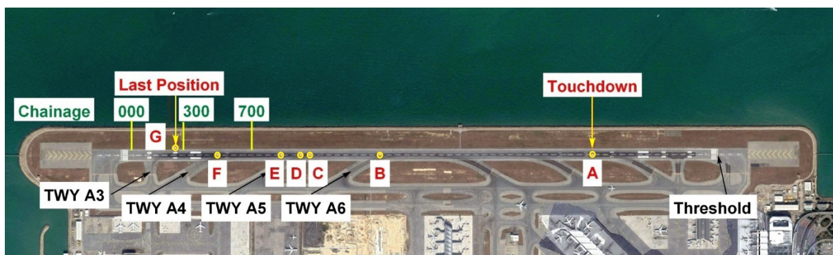
Figure 11: Critical Points of the Rollout
