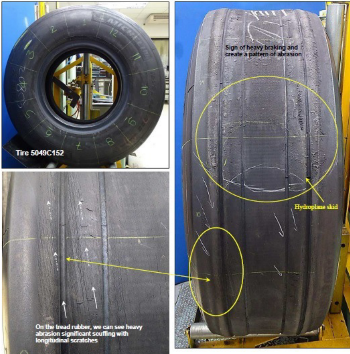
Figure 21: Damage on No.2 Tyre
