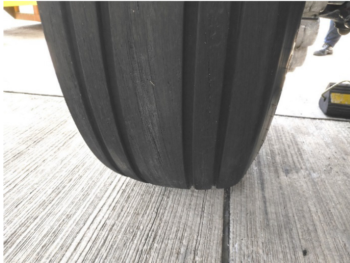
Photo 5: Significant Longitudinal Scratch Marks on No. 4 Tyre
